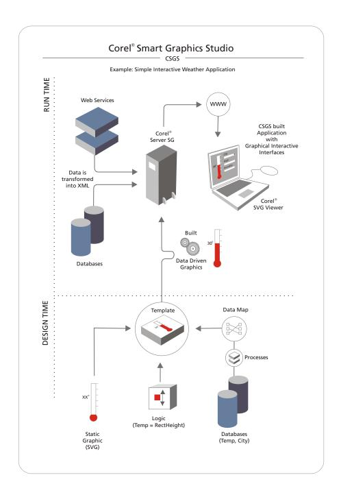
This picture shows how the Corel Smart Graphics Studio components are integrated into a workflow. It shows the workflow that a designer would use to transform a static graphic of a thermometer into a smart graphic driven by data from a Web service.
